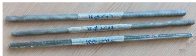
Fig. 3. Locally produced HGFRP bars.
