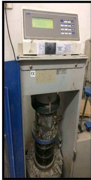
Fig. 2. Concrete cubes testing.
